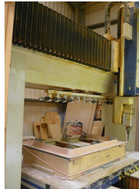
5-AXIS CNC MACHINING CENTRE TRIMMING WINDOW MOULDINGS ACCURATELY AND CONSISTENTLY
